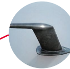
Pitot tube (total pressure)
